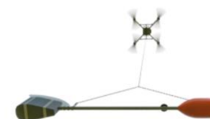
Survey with a UAV equipped with quantum magnetometer
